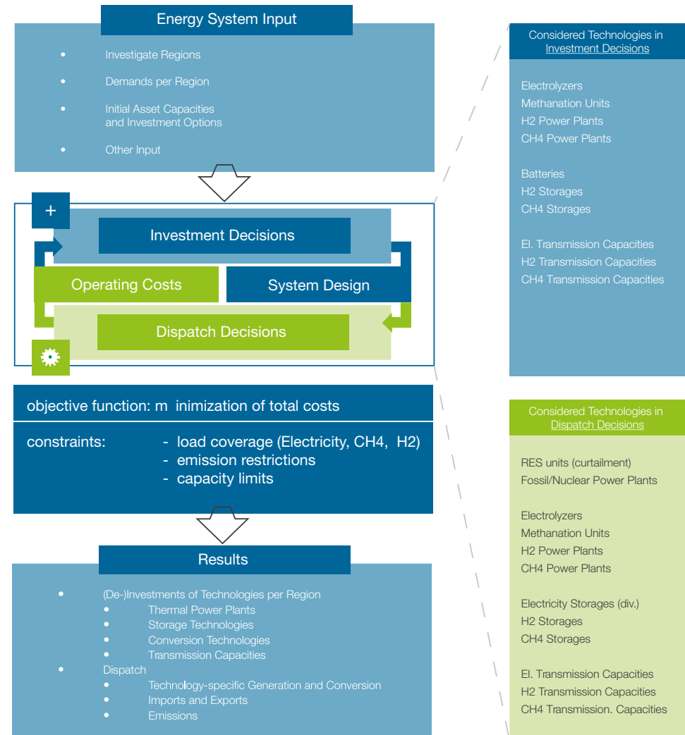
Figure 9: Overview of developed integrated system expansion model
